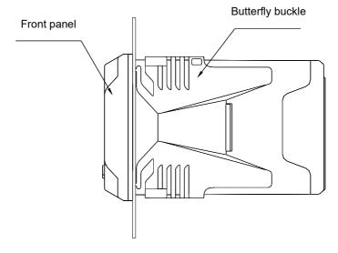
Figure 3 Schematic diagram of meter installation
