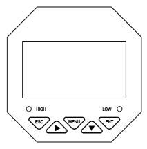
Figure 6 Button distribution diagram
