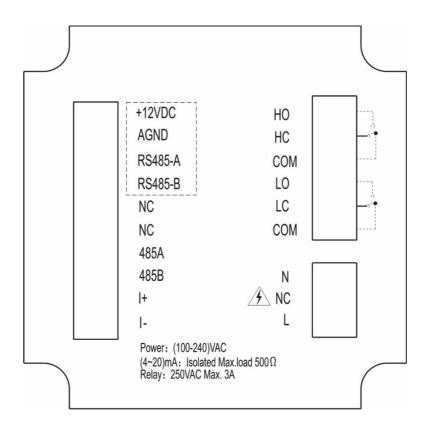
Figure 4 220VAC wiring diagram
