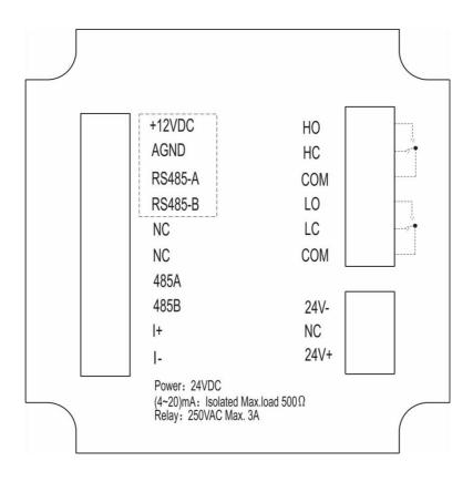
Figure 5 24VDC wiring diagram
