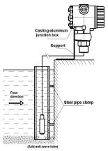
When measuring liquid level in a fluid with large fluctuations, it is recommended to add damping devices as shown in the figure to reduce the impact of fluctuations on liquid level measurement, and to fix the cable and junction box at the outlet.
