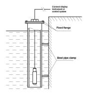
In the measurement of still liquid, the level transmitter can be directly put into the liquid, and the cable and junction box can be fixed at the outlet.
