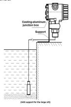
When measuring the still liquid in an open container, the level transmitter can be directly put into the bottom of the container and the cable and junction box can be fixed at the opening of the container.
