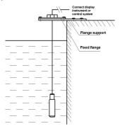
When measuring the liquid level in the flowing liquid, insert a steel pipe with an inner diameter of about Φ 30mm in the liquid, and open two to three holes of about Φ5mm in the high and low positions of the pipe in the reverse direction of the liquid flow to allow the liquid to enter the pipe easily, and the cable and junction box are fixed at the outlet.
