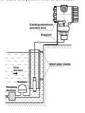
In the liquid level measurement with large silt, it is necessary to install the mounting bracket to prevent the silt from blocking the pressure hole and causing test errors
