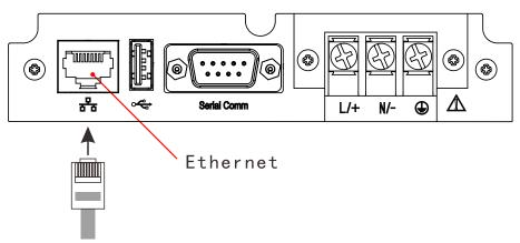
Use network cable connector to connect RJ45 connector.
